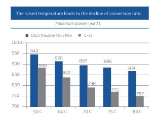
The operating temperature of module is basically larger than the standard test temperature 25 C data possibly reaching 60 C in summer). The flexible thin film module is low in temperature coefficier and prominent in high temperature performance.
